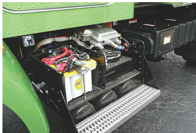
In a box behind the driver's steps are the chassis battery (left) and Eaton electronic controls with a horizontally mounted cooling fan. Orange cables carry 340 volts to and from the motor-generator and lithium-ion batteries, in the large black box to the rear.
