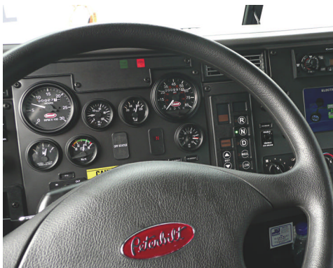
A color screen on the dash, next to UltraShift selector, shows what mode the hybrid system is in and whether it's charging or proceeding on electric or diesel power.
