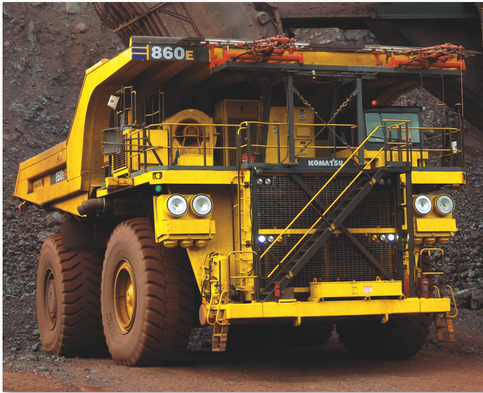
Komatsu's new 860E-1K mining truck features a 2,700-horsepower, 16-cylinder, two-stage turbocharged diesel that meets Tier 2 emissions requirements.
