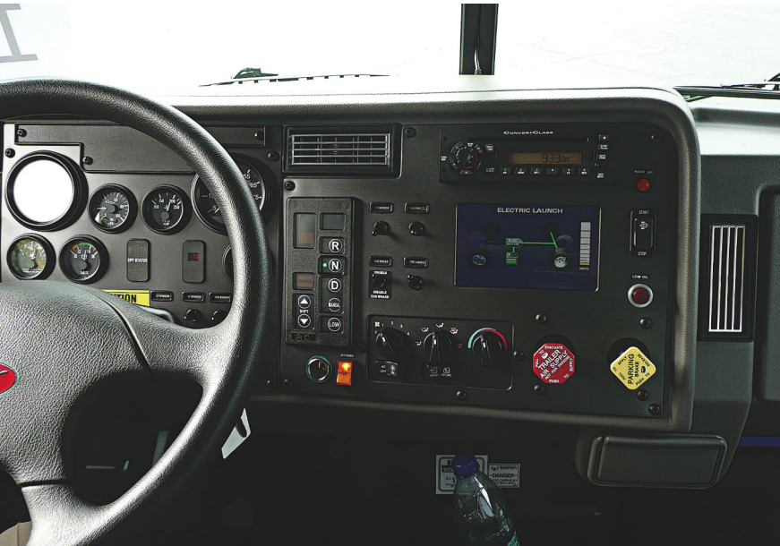
A color screen on the dash, next to UltraShift selector, shows what mode the hybrid system is in and whether it's charging or proceeding on electric or diesel power.
