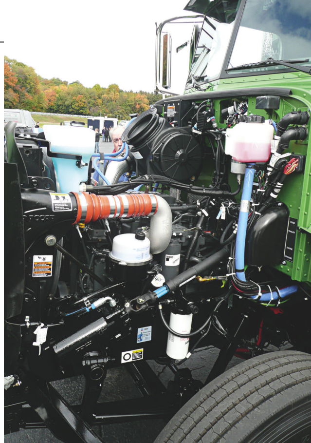
The 300-horsepower Paccar PX-6 diesel works with Eaton hybrid system's 60-horsepower electric motor to launch the truck, and it handles most or all propulsion at higher speeds.
